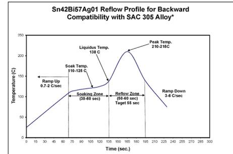
\*This profile is simply a guideline. For a reliable solder joint the reflow profile must product homogeneous mixing of the Sn42Bi57Ag01 alloy with the SAC305 component sphere. The mixing level between the Sn42Bi57Ag01 and SAC305 alloy is a function of reflow peak temperature, time above liquidus, component size and sphere alloy. Your optimal reflow profile may be different from eh one shown based on your oven, component sphere size and sphere alloy.
