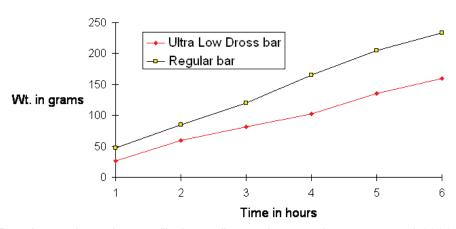
Results are based on an "in-house" experiment using an aerated 2000 gram solder pot at 260 °C (500 °F).
