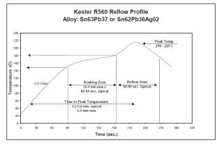
The recommended reflow profile for R560 made with either the Sn63Pb37 or Sn62Pb36Ag02 is shown here. This profile is simply a guideline.
