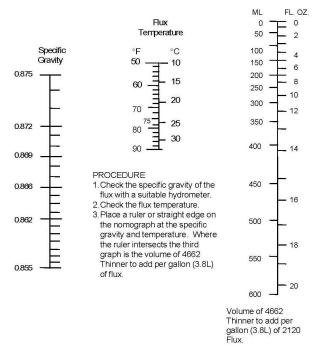
Checking the specific gravity at regular intervals and adding the appropriate amount of Kester 4662 Thinner will assure consistent, controlled soldering results. Use of the Flux control nomograph simplifies determination of the correct amount of thinner to add to return the flux to its correct specific gravity.
