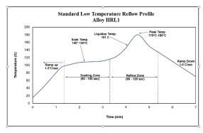
The general recommended convection reflow profile for the NP510-LT HRL1 is shown here as a starting point. Your final profile will depend on your board mass and component combination. NP510-LT HRL1 has excellent solderability and wetting capabilities in air or nitrogen reflow atmospheres reflow equipment. Your optimal profile may be different from the basic graph. Please contact Kester Technical Support if you need profiling advice.
