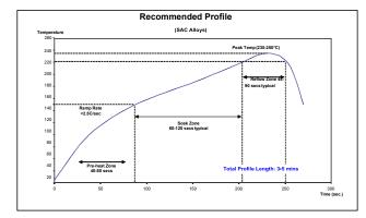
The general recommended convection reflow profile for NP505-HR formula made with SAC and Innolot alloys is shown here as a starting point.
