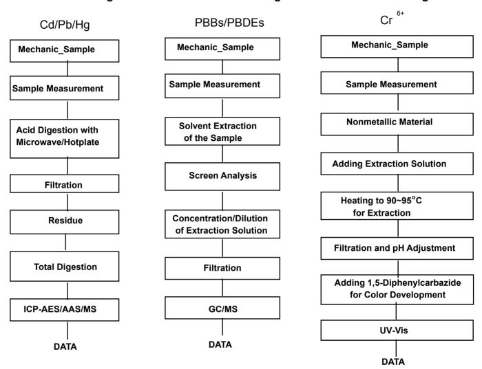
The samples were dissolved totally by pre-conditioning method according to above flow chart for Cd,Pb,Hg. Section Chief: Gilsae Yi
