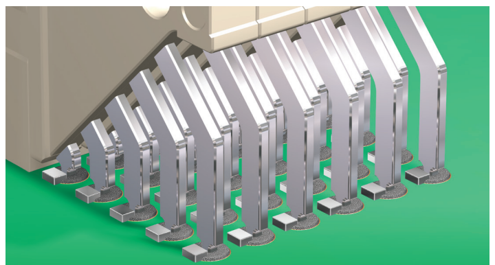
Solder paste and preforms reflowed
