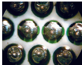
Solder paste and preforms reflowed
