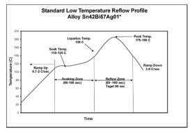
The general recommended convection reflow profile for the NP505-LT formula made with Sn42Bi57Ag01 is shown here as a starting point. Your final profile will depend on your board mass and component combination. NP505-LT has excellent solderability and wetting capabilities in air or nitrogen reflow atmospheres reflow equipment. Your optimal profile may be different from the basic graph. Please contact Kester Technical Support if you need profiling advice.
