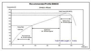
The recommended reflow profile for EM808 made with SAC alloys is shown here. This profile is simply a guideline. Since EM808 is a highly active solder paste, it can solder effectively over a wide range of profiles. Your optimal profile may be different from the one shown based on you oven, board and mix of defects. Please contact Kester Technical Support if you need additional profiling advice.
