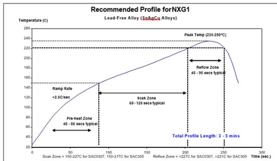
The recommended reflow profile for NXG1 made with SnAgCu alloy is shown here. This profile is simply a guideline. Since NXG1 is a highly active solder paste, it can solder effectively over a wide range of profiles. Your optimal profile may be different from the one shown based on your oven, board and mix of defects. Please contact Kester Technical Support if you need additional profiling advice.
