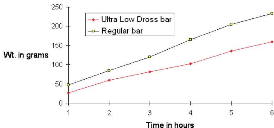
Results are based on an “in-house” experiment using an aerated 2000 gram solder pot at 260 °C (500 °F).
