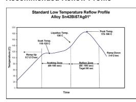
The general recommended convection reflow profile for the NP505-LT formula made with Sn42Bi57Ag01 is shown here as a starting point. Your final profile will depend on your board mass and component combination. NP505-LT has excellent solderability and wetting capabilities in air or nitrogen reflow atmospheres reflow equipment. Your optimal profile may be different from the basic graph. Please contact Kester Technical Support if you need profiling advice.
