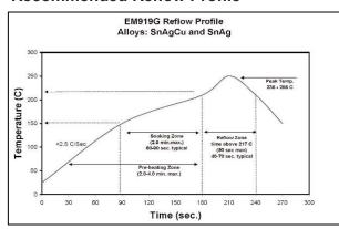
The general recommended convection reflow profile for EM919G formula made with typical lead free alloys is shown here as a starting point. Your final profile will depend on your board mass and component combination. EM919G has excellent solder-ability and wetting capabilities in air or nitrogen reflow atmospheres reflow equipment. Your optimal profile may be different from the basic graph. Please contact MacDermid Alpha Technical Support if you need profiling advice.
