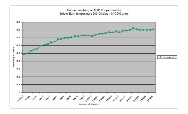
This shows an average leaching rate of 0.01% Cu per 1,000 boards. Each process is unique, and this is an indication only of the leaching rate (based on actual data).
