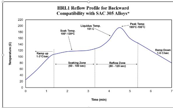
The general recommended convection reflow profile for the NP510-LT HRL1 is shown here as a starting point. Your final profile will depend on your board mass and component combination. NP510-LT HRL1 has excellent solderability and wetting capabilities in air or nitrogen reflow atmospheres reflow equipment. Your optimal profile may be different from the basic graph. Please contact Kester Technical Support if you need profiling advice.
