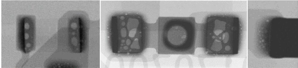
**Large voids:** For the large voids underneath the component, this is most often caused by outgassing of the solder paste flux. In this case, flux did not have time to escape from underneath the component body. This is quite common and is nearly impossible to fully eliminate without the use of reflowing in vacuum.
