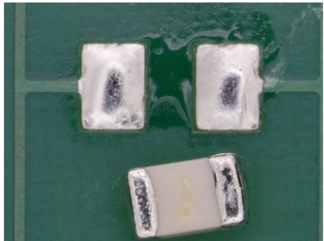
Figure 9: Flux Accumulates Under Bottom Terminations
