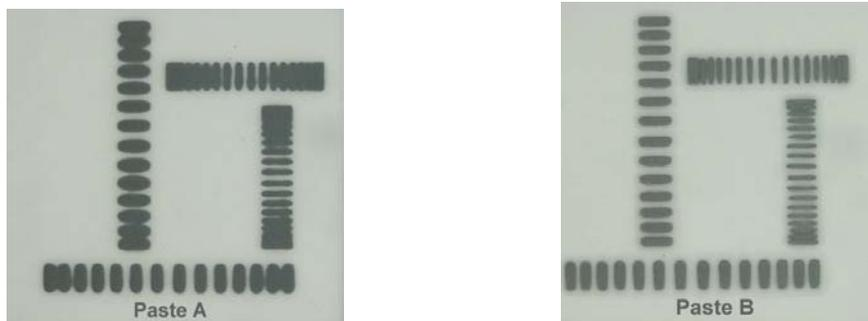
Both pastes were run through a reflow oven at 180°C. Paste B has better hot slump properties than Paste A and would less likely cause bridges, solder balls or mid-chip balling. For fine pitch components it is critical to select a lead-free paste with a heat stable gelling agent.
