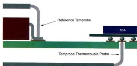
A test board is essential for the first lead-free assembly to insure thermal requirements are met across the board. The diagram to the left, shows the proper way to measure the heat applied to the balls in the grid array.
