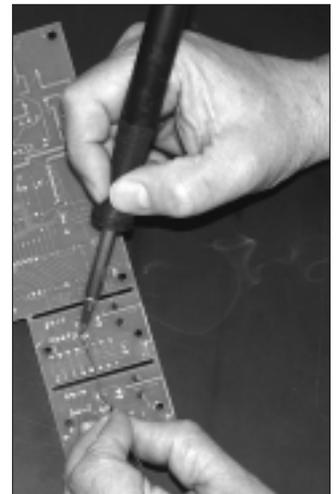
to thermally equalize the assembly, and the second is to activate the flux. Activating the flux essentially allows the paste flux to “chemically scrub” the surface oxidation of the surface finishes on the printed circuit
