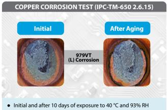
Minor corrosion was observed on the test panels without pitting of the copper, classified under "L" category as per J-STD-004 or "M" category as per J-STD-004B.
