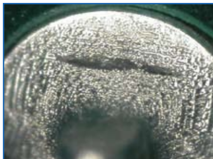
Figure 2. SAC305 Wave Soldered Joint Top-side.
