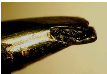
Lead-free tip failure after 3 weeks
