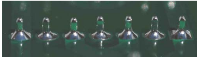
Figure 6. Bottom-side solder joints
