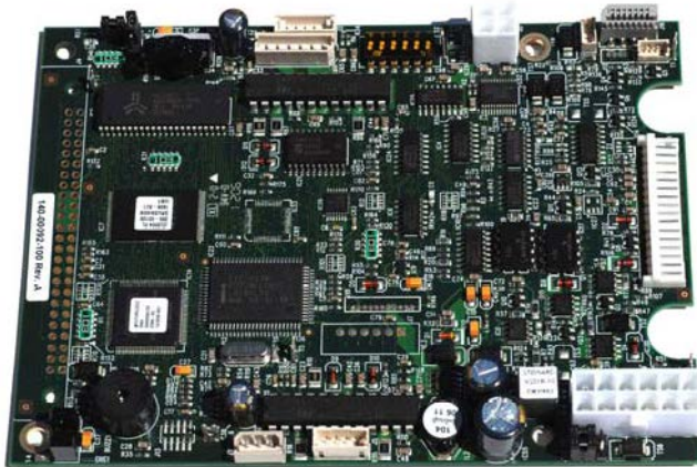
Figure 4. K100LD and SAC305 PCB Board soldered with SAC305 solder paste, K100LD wave solder and K100LD wire solder. Water soluble fluxes were used.
